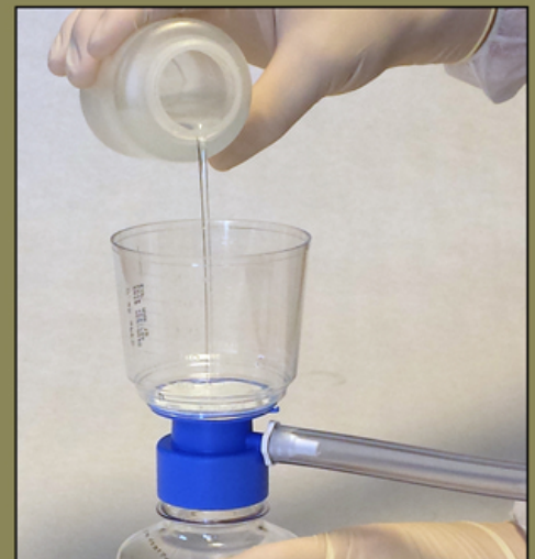
After area of interest is swept for DNA, pour the collected buffer solution through the filter, seal filter and send to lab for analysis.
