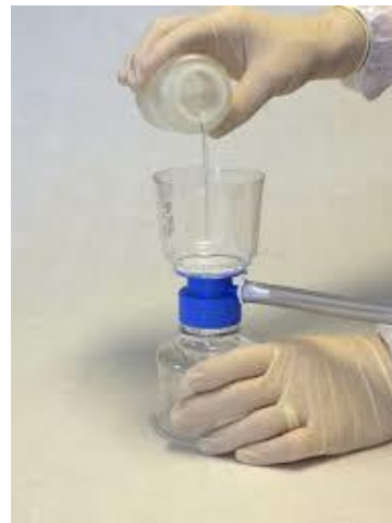
Buffer containing suspended particles, including the DNA contained from the pants' pocket, is poured through a sterile filter where the biological material will bind to the filter and become concentrated.
