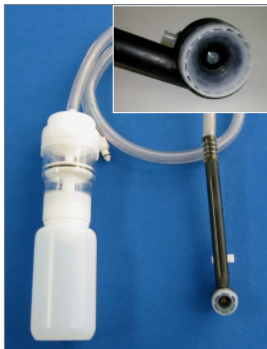
Figure 1: LRTC with filter assembly and small sampling head; insert: large sampling head; both prototypes
